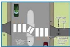
Typical Mid-Block Road Crossing with Median Refuge
